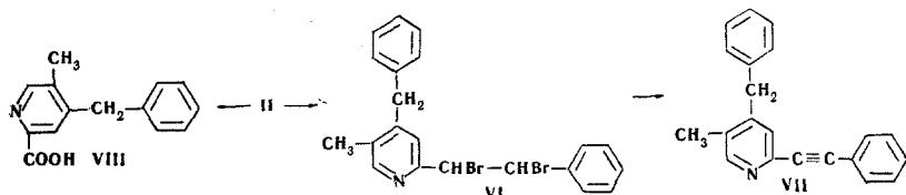
An attempt was made to oxidize II at the ethylene group, the oxidation being carried out with potassium permanganate in acetone at  $0^\circ$ . It is a characteristic of this reaction that it affords readily-isolable benzoic acid, which was isolated in 45% yield. 5-Methyl-4-benzylpyridine-2-carboxylic acid (VIII) was isolated both in the free state and as its ethyl ester.
